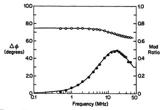
Fig. 4. Differential phase ( $\bullet$ ) and modulation ( $\circ$ ) data for HRP(desFe); experimental conditions the same as in Fig. 3. Solid curves correspond to values obtained for the best-fit analysis of phase and modulation data;  $\rho_1 = 86$  ns,  $\rho_2 = 12$  ns,  $a_1 = 0.163$ ,  $a_2 = 0.005$ .
