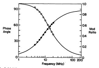
Fig. 2. Multifrequency phase (•) and modulation (•) lifetime data for HRP(desFe) in 0.1 M phosphate buffer (pH 7.4). Solid curves correspond to a single exponential decay of 16.87 ns. Excitation wavelength was 514.5 nm; emission was observed through a Schott OG 570 cuton filter which passes λ > 560 nm.
