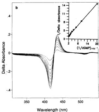
**Figure 2.** Panel a: optical absorption spectra of T4MPyP in the absence (I, top) and presence (II, bottom) of dGMP. Porphyrin concentration is  $10~\mu\text{M}$  dGMP, 2~mM in 100~mM phosphate buffer, pH 7.1. Spectra were obtained using a 1 cm quartz optical cell. Panel b: absorption difference spectra of T4MPyP ( $10\mu\text{M}$ ) titrated with dGMP (final concentration 0.47 mM). Inset is a fit for eq 1 for 1:1 association stoichiometry of the complex.
