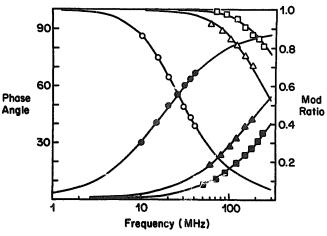
Fig. 1. Multifrequency phase (closed symbols) and modulation (open symbols) data for  $10^{-5}$  M NADH in buffer (squares),  $10^{-5}$  M NADH plus  $10^{-5}$  M mMDH dimer (triangles) and  $10^{-5}$  M NADH/ $10^{-5}$  M mMDH plus  $10^{-2}$  M hydroxymalonate circles). The buffer was 50 mM Tris-HCl (pH 7.4) (25°C). Solid lines correspond to calculated curves with component lifetimes and fractional intensities as indicated in the text.
