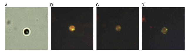
Fig. 3. Wide field epifluorescence images of *Nannochloropsis* sp. cells infused with Nile Red. (A) shows the cell under bright field microscope at 100×. (B–D) show cells after addition of Nile Red. (A) Bright field (100×), (B) after 2.5 min. (C), after 10 min, (D), after 19 min.
