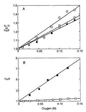
Figure 1. (A) Intensity (□), phase lifetime (○) and modulation lifetime (●) quenching of the porphyrin emission of HRP(desFe) by oxygen. Intensities and lifetimes were measured through an OG 570 cuton filter and excited at 514 nm at 20°C. (B) Intensity quenching of hemoglobin-(desFe) (■) compared to HRP(desFe) (□).
